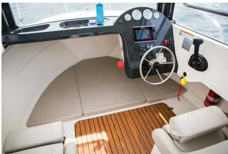
the self draining deck ensures water disperses quickly keeping the deck dry.
