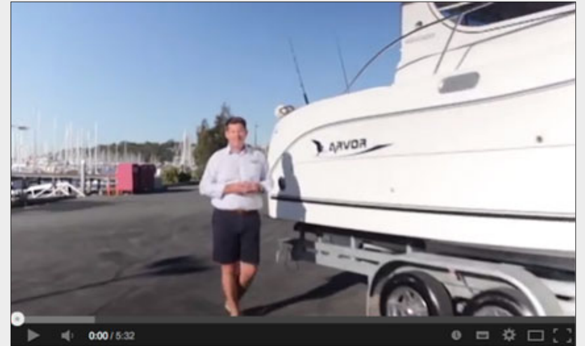
Above: Brisbane-based Crawford Marine's Matt Hodson presents a very good Aussie video they produced (on Moreton Bay) which apart from showing off the Weekender very nicely, also reminds us that although this rig is over-width (2.78m instead of 2.5m) it is easily towed with a standard overwidth towing kit - flags, signs and flashing lights, as it is only about 3.5t all up.
