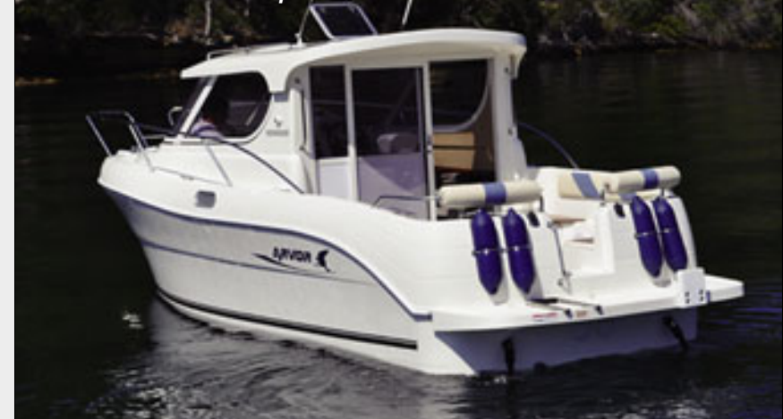
A couple of interesting shots (Above) The transom 'pocket' shape (lowers the draft, gives better water flow for the prop, straighter tracking) and (Below) at rest with a couple of blokes forward. Off plane vision is excellent.
