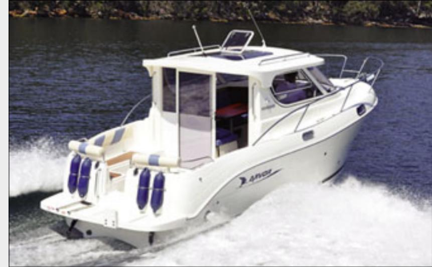
**A couple of interesting shots (Above) The transom 'pocket' shape (lowers the draft, gives better water flow for the prop, straighter tracking) and (Below) at rest with a couple of blokes forward. Off plane vision is excellent.**
