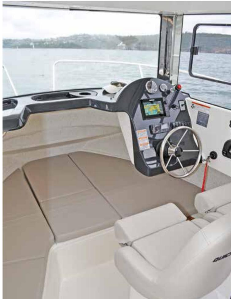
Above: The wheelhouse layouts are similar for both boats with full protection and excellent visibility. This 690D had a chartplotter/fishfinder and trolling valve on the dash. The forward cushions of both Arvors extend to double-berths with infill sections.
